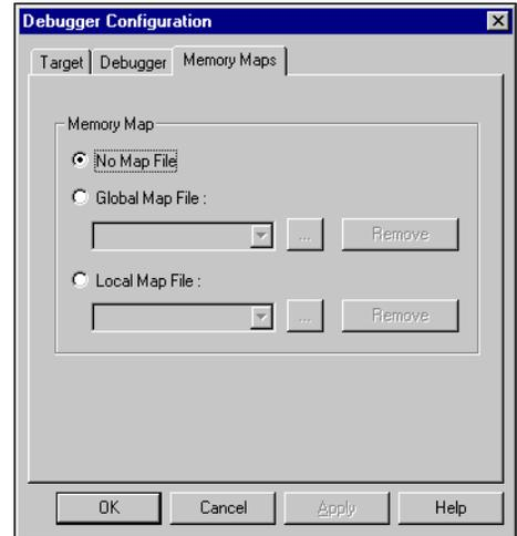
**Figure 9-11 Configuration of ARM Debugger memory maps**
